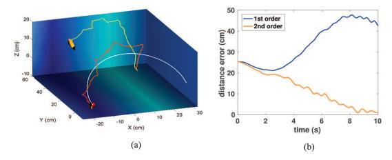
Fig. 13. Tracking performance of the same system in the presence of +10 cm/s  $\hat{y}$  fluid drift. The yellow system corresponds to first-order needle variation actions; the red system corresponds to second order. The target trajectory (red ball) is indicated with white traces over a 10-second simulation. Figure 13b shows the error distance as a function of time, clearly demonstrating the advantage of the second-order approach. Animation of these results is available in Extension 4.
