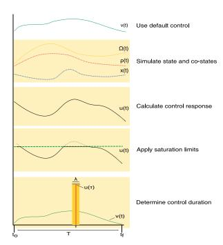
**Fig. 2.** The steps of the controller outlined by Algorithm 1. Using the default control, the states and co-states are forward-simulated for the time horizon  $[t_0, t_0 + T]$ . The optimal control response is computed from (11), and saturated appropriately. At the end, the algorithm determines the finite duration of the inserted single action, evaluated at an application time  $\tau$ , with a line search.
