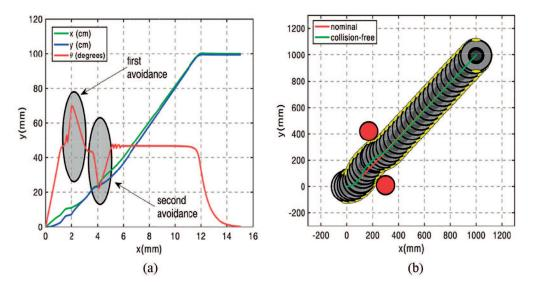
**Fig. 6.** (a) Differential drive using second-order needle variation actions in the presence of obstacles. (b) The deviation from the nominal trajectory that is the solution to the no-obstacle task. The system performs two maneuvers to avoid each obstacle. These are evident in the angle deviation (compare with Figure 3c).
