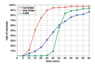
**Fig. 11.** Convergence success rates of first- and second-order needle variation controls ((12) and (11), respectively) and iLQG for the underactuated *dynamic* vehicle model. Simulation runs: 280.
