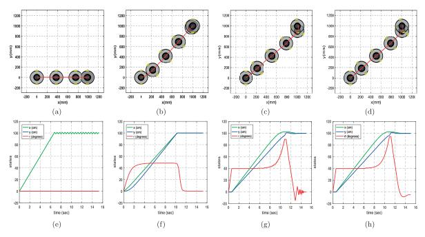
**Fig. 3.** Differential drive using first- and second-order needle variation actions, iLQG, and DDP, from left to right. Snapshots of the system are shown at t = 0, 2.5, 5, 7.5, 10, and 12.5 s. The target state is  $[x_d, y_d, \theta_d] = [1000 \text{ mm}, 1000 \text{ mm}, 0]$ .
