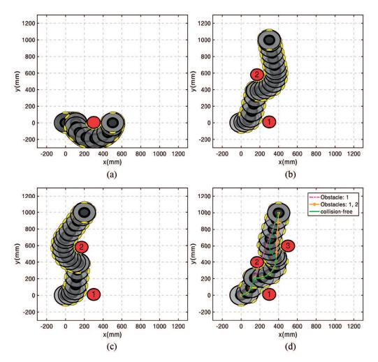
**Fig. 7.** Trajectories of the differential drive in the presence of obstacles. Figure 7d shows a comparison of the solution to the trajectories generated when considering only a) obstacle 1 and b) obstacles 1 and 2, both of which collide with the obstacles. Simulations run in real time in MATLAB.
