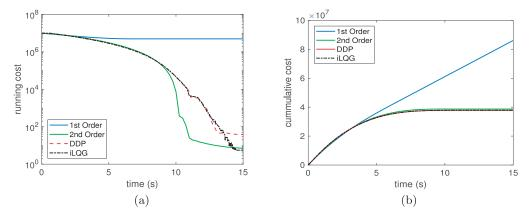
**Fig. 4.** (a) Plot of the running state cost and (b) plot of the integrated (cumulative) cost, including the control cost. DDP and iLQG obtain the same cumulative cost, with slightly different trajectories (see Figure 3). Second-order needle variation actions demonstrate improved convergence to the target over DDP and iLQG, despite optimizing over one single action at each iteration.
