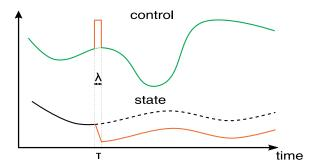
Fig. 1. A fixed-value perturbation in the nominal control, introduced at time  $\tau$  and with duration  $\lambda$ , and the associated variation in the state. In the limit  $\lambda \to 0$ , the control perturbation becomes a needle variation.
