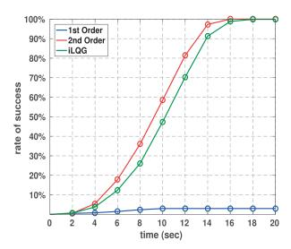
**Fig. 5.** Convergence success rates of first- (12) and second-order (11) needle variation controls for the kinematic differential drive model. Simulation runs: 1000.
