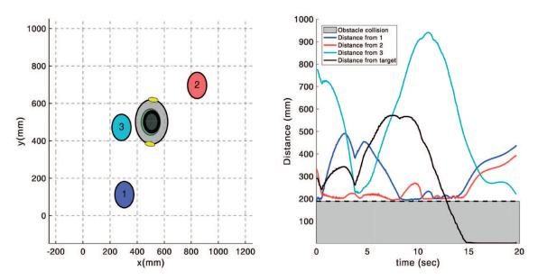
**Fig. 10.** Performance of second-order needle variation actions in the presence of three moving obstacles. The left figure shows a snapshot of the simulation; the right figure plots the distance of the agent from each object and the target, where the gray area indicates the threshold minimum distance to avoid collision with the obstacles. The controller converges to the target in a collision-free manner (the simulation runs in real time in MATLAB). For visualization, see Extension 2.
